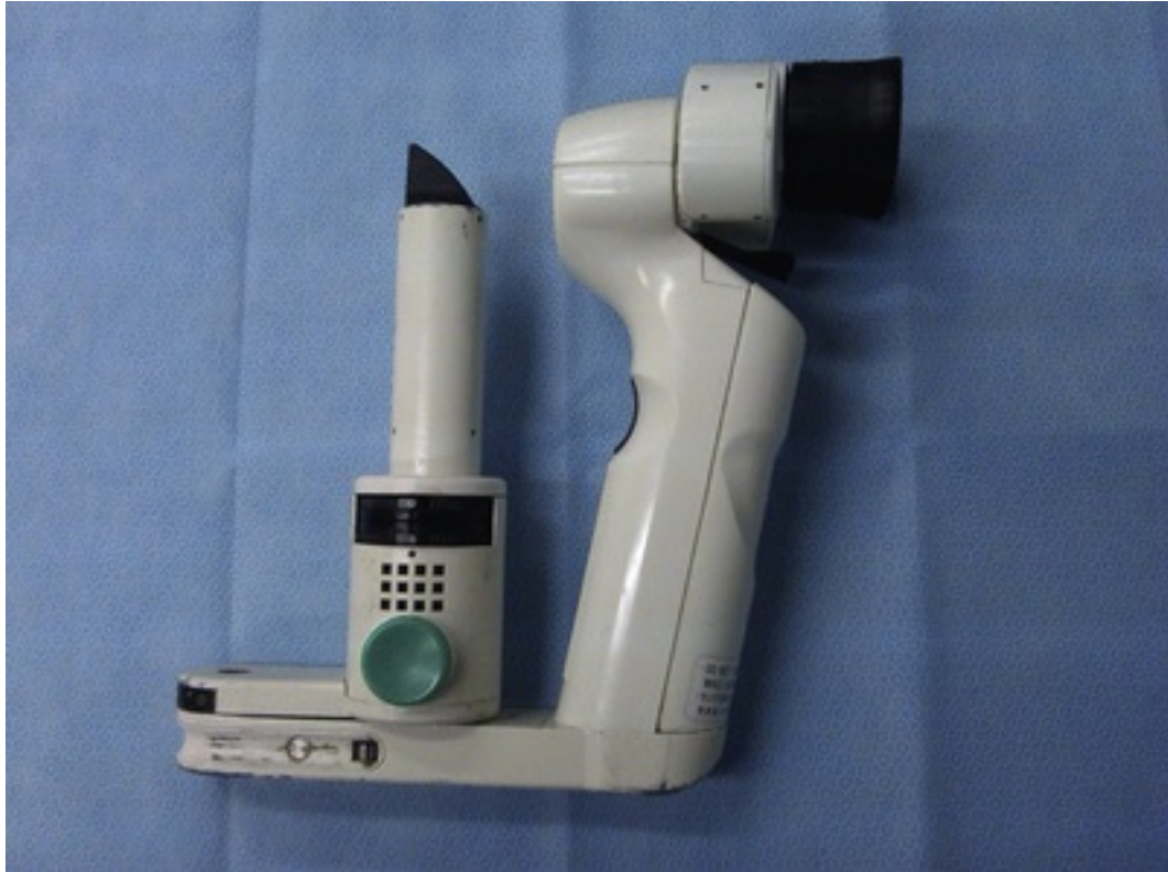
FIGURE 11-1 Slit lamp biomicroscope, which provides illumination and magnification when evaluating the anterior segment of the eye.
