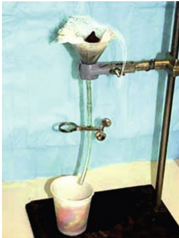
E-FIGURE 242-3 Baermann fecal sedimentation requires only simple equipment: a stand, a funnel, tubing, a collection vessel, and a clamp.
